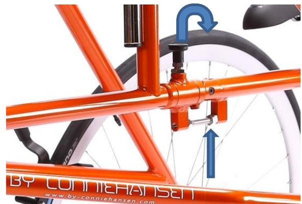
**Remember:** Make sure that the user doesn't catch clothes or skin between the stop bolts in the drop down link.
