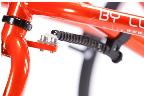
An open spring system is used on PETRA size 0 and 1. It can also be used on size 2.
