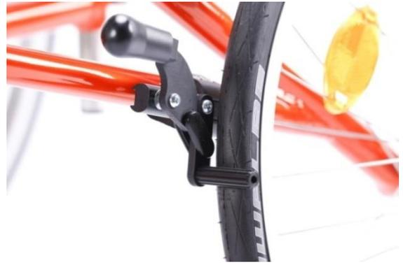
The brake arm and the clamp can be mounted with a 5 mm Allen key. The cleat and the cylinder on the claw must sit fairly straight or perpendicular to the tyre. The distance should be approx. 5 mm when the brake is open and the tyres are well pumped.
