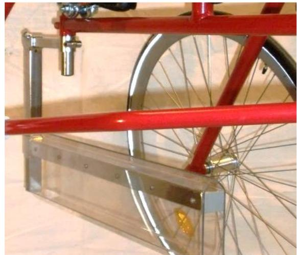
The plate mounted with a square-sectioned post from the seat post and a vertical square-sectioned post down to the plate.
