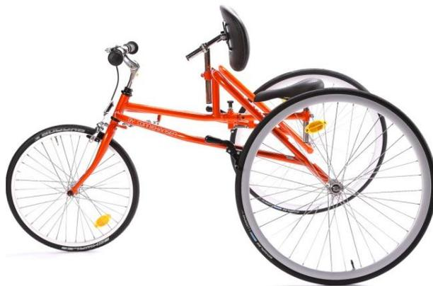
The saddle's position over the rear axles and the user's weight and position are essential for tip-point and stability. The saddle's back edge must not be more than 2-4 cm behind the rear axles. The saddle post must turn forwards to secure stability. Adjust the angle and the distance between saddle and chest plate to fit the user.
