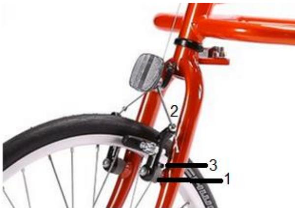
The cantilever brake is normally for size 0 and 1 but it can also be used on size 4. The brake levers are mounted on pivots on the fork's leg. In the bottom there is 1) a small spring and a pin for adjustment of the tension. 2) The brake's cables must be fairly tight and well balanced to work. Their
