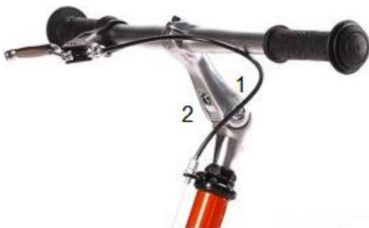
1) The handlebar stem can be turned both ways and adjusted in height with a 6 mm Allen key in the bolt on top. 2) The angle on the top part of the stem
