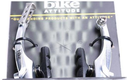
The V-brake levers are placed on pivots and their tension is decided by the spring in the bottom and the pin's position. The cable must be mounted with a fitting tension 1) in the top of the brake lever. Fine tuning can be done 2) on the site of the brake levers.
