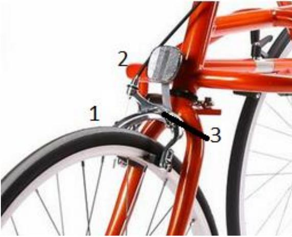
Racing brake for Size 2, 3 and 5 is mounted at the top of the front fork. Adjustment of the brake levers' opening can be done by: 1) Pulling the cable. 2) Adjusting the adjustment screw. 3) There is a small Allen screw on top of the brake to adjust the balance between the openings of the two claws. 4) The braking blocks have to sit tightly and directly into the rim.
